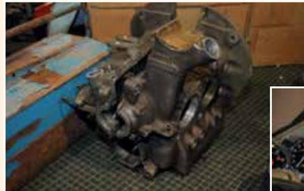
◀ How about a 30hp engine crankcase? You can tell it's an industrial application by the 122 engine number
